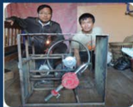
Hydro powered water pumping device
